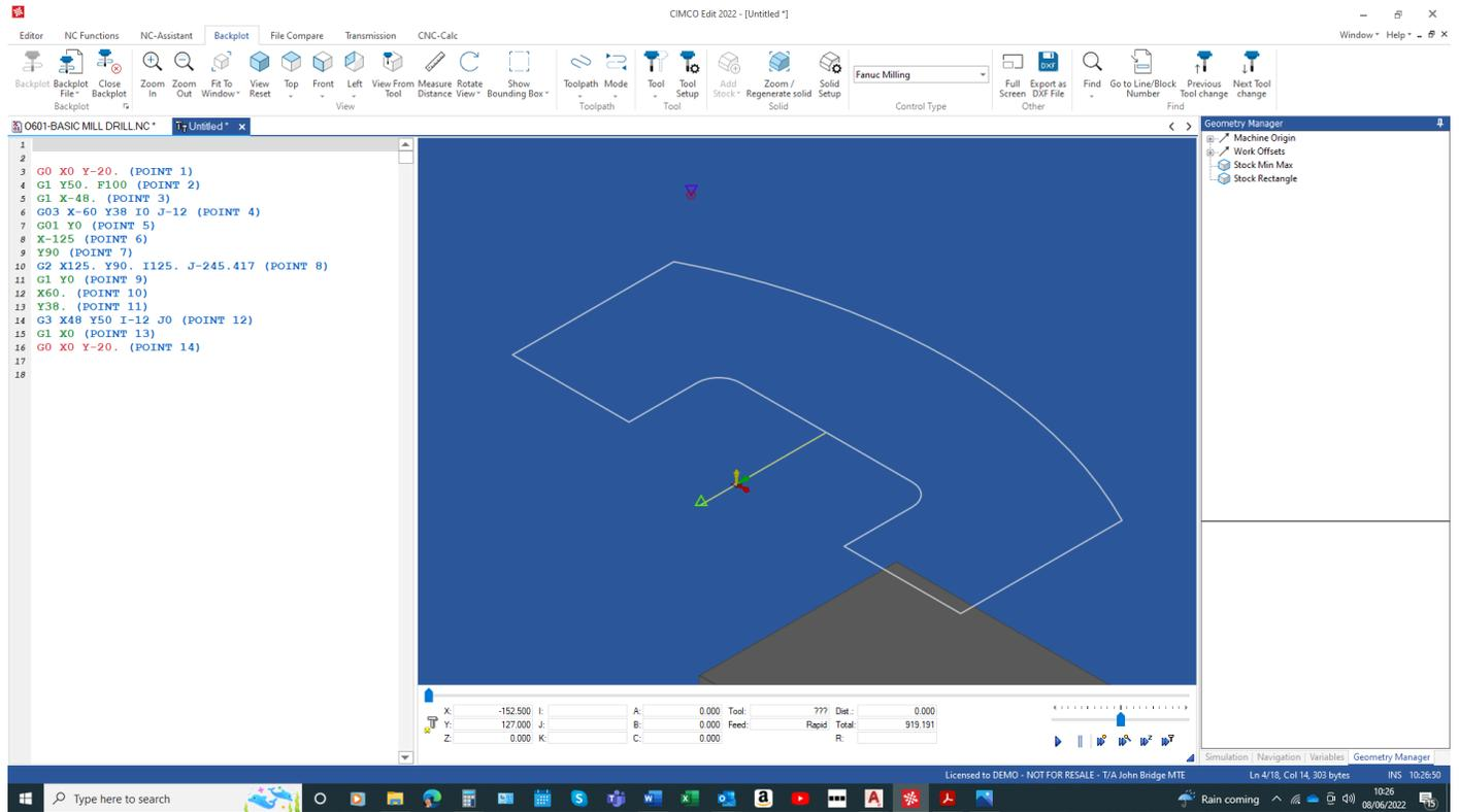
A further reminder - do not forget to change from circular to linear from element to element as the profile changes. All group 1, move commands are modal e.g., after a G02 block if you were to enter X Y coordinate the CNC control will still try to move circular unless you place a G01 at the start of the block to define that this move is now linear.
