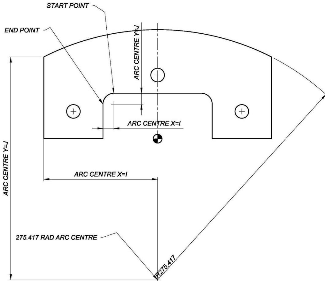
We have already entered the start point 3 and we are going to point 4 in a counterclockwise direction the block will start
