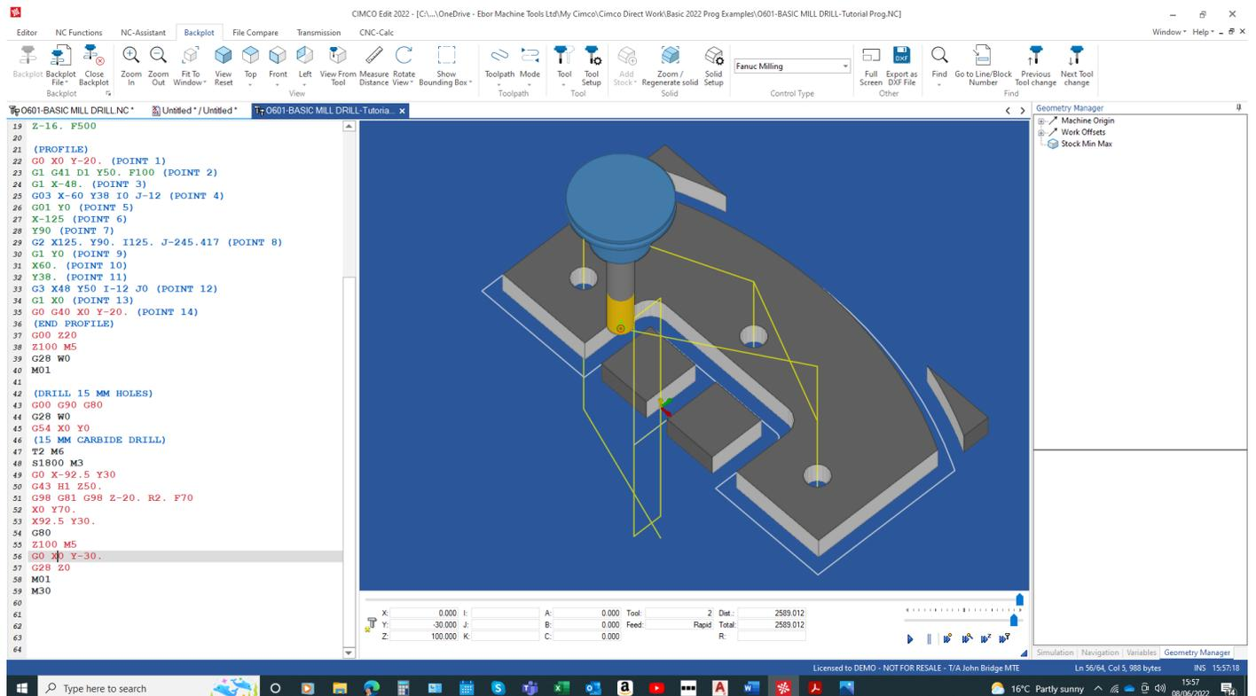
Here is a full copy of the program for you to check yours against. This program should run on most CNC machines with Fanuc or Haas CNC controls. There may be a small amount of editing to do from machine-to-machine dependent on the Machine Tool Builders application of the CNC control. The edits will apply generally to the header and trailer format and syntax.
