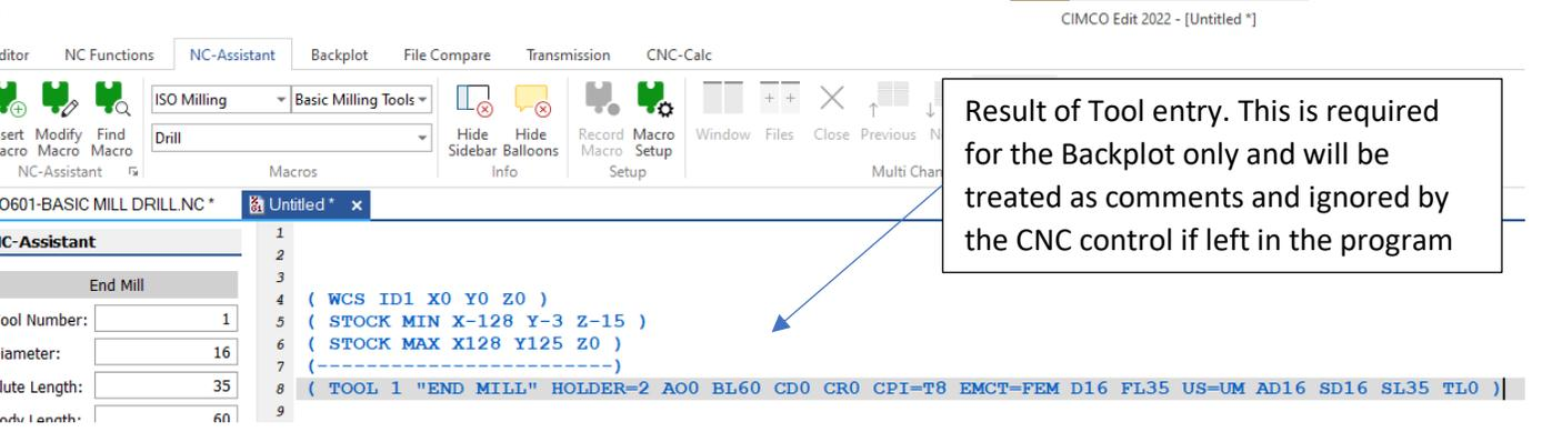
We also need to set a machine origin for the Z axis otherwise the Tool Change will place the Tool holder flange at Z0 in Backplot and it will look as though the Tool is buried in the Stock. The size of the origin should be a little longer than the longest tool and this will lift the Tools above the job in Backplot. On a CNC machine this is all taken care of by the Machine Coordinates, Work Shifts, and Tool Length offsets.
